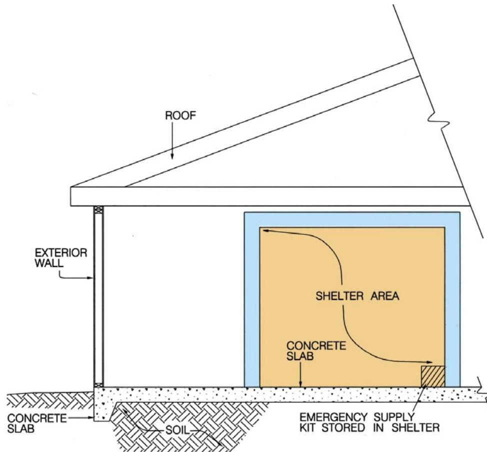
susceptible to the impact of missiles, it should not be built of wood framing. Instead, it should be built of concrete or concrete masonry. Access to this type of shelter can be provided through an existing door or window in an exterior wall of the house.
